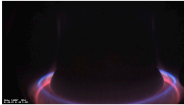
Figure 2.5: Visible light camera image of an XPR in AUG discharge (#40007) at 3.4 s, showing the blue light above the x-point mainly from N^{2+} and the red light of Balmer radiation at the divertor legs, adapted from figure 1 in [3].
